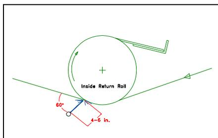
Forming fabrics are far too often taken off due to poor operation caused by plugging with contaminants and fibers which could have been removed with efficient, high pressure, needle shower cleaning.
