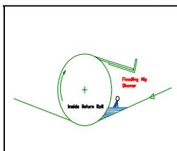
The theory behind the flooded nip shower is to force a large volume of water between the fabric and an internal roll. The action of the nip will create a considerable hydraulic force that will push the water through the fabric.
