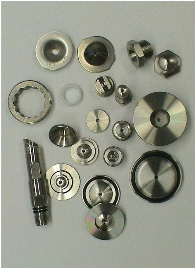
Synthetic industrial jewels in the form of white sapphire and red ruby can increasingly be found on high pressure shower applications on most modern paper machines throughout the world. Longer life of the nozzle orifice and more importantly a longer lasting laminar jet during the life of the nozzle is typically the driving force for choosing a synthetic sapphire or ruby orifice nozzle in lieu of a solid 316 stainless steel body nozzle.
