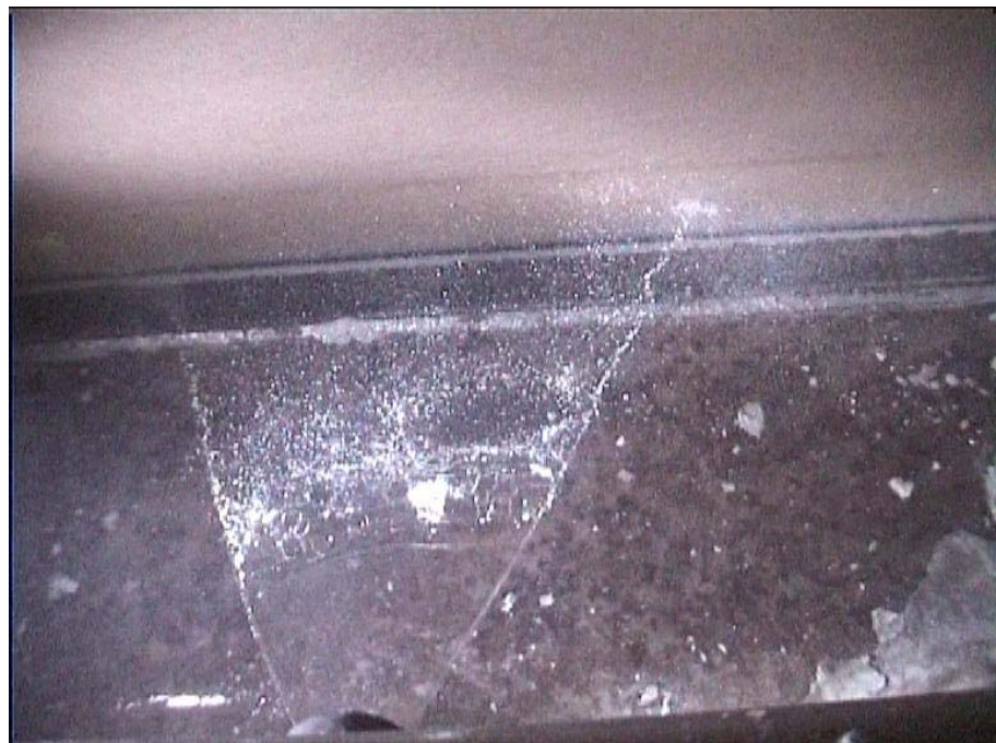
Picture 21: streaky water application by non uniform fan jets
