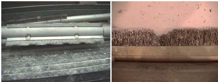
Picture 10: deformed bristles due to nozzle shape
